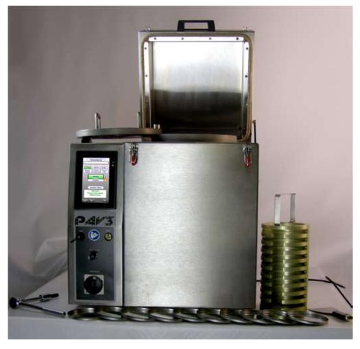
The Next Generation of an Innovative System for Simulated Aging of Asphalt Binder
