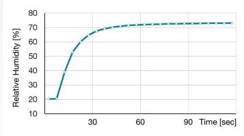
Two factors reduce the leap frogging time immensely: The small air volume of the measuring sleeve and the extreme fast reaction time of the probe.
