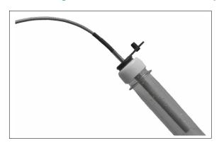
The humidity standard tube allows a fast and easy on-site functional and calibration check of the instrument and the in-situ probe as recommend by ASTM.
