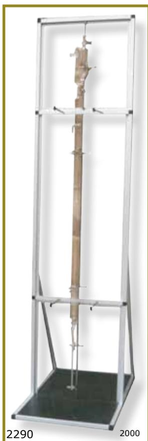
Consisting of: adsorption column with upper female tapered linkage and male tapered cap equipped with connection, structure made of aluminum.
