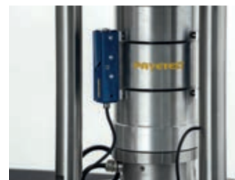
B203 verification device with on-specimen B200-01 LVDTs and load cell
