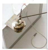
Crucible holder made in stainless steel keeps the cup assembly ready to use.
