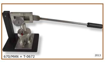
680/1/4 1/4 SCALE GREASE WORKER ASTM D1403
