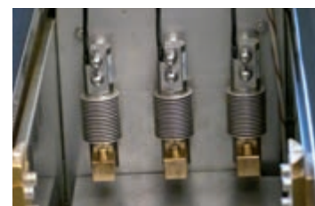
Detail: 3 load cells 500 N
