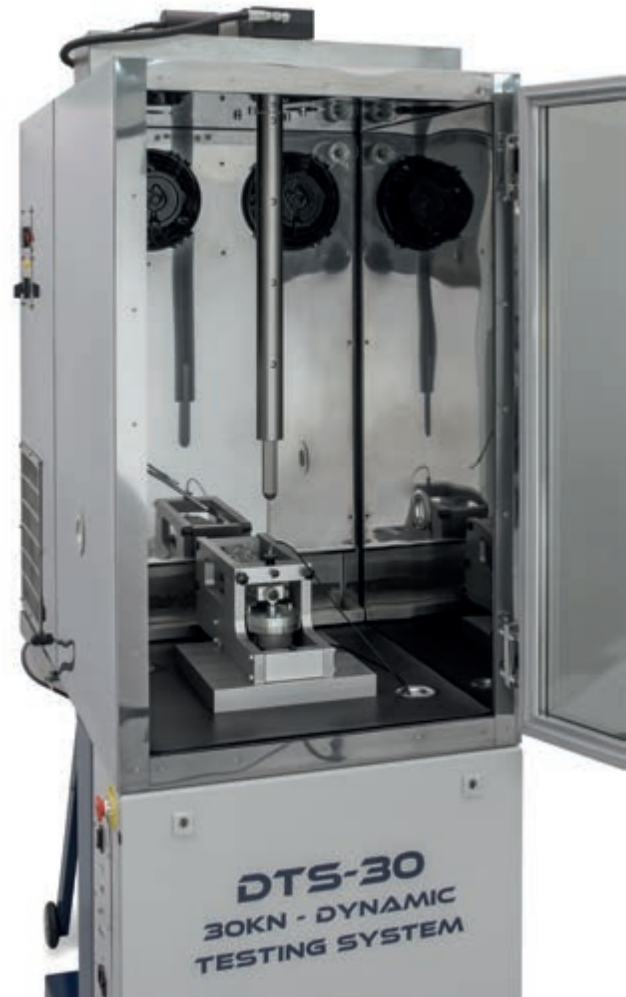
B230 DTS-30 Dynamic Testing System, open
