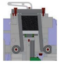
During the compaction process a lateral displacement is applied to the specimen along with a vertical load, which results in a shearing action that makes the compaction similar to the the on-field one.
