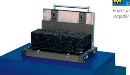
Specimen is extruded after the machine has completed the specified number of cycles, or when the required specimen height has been reached.
