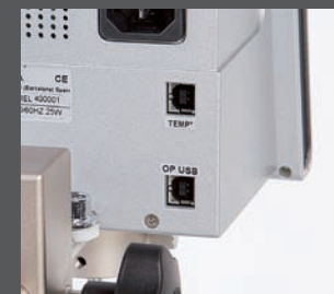
Rear view to the viscometer showing the new USB interface that provides a faster transfer of data to the computer.
