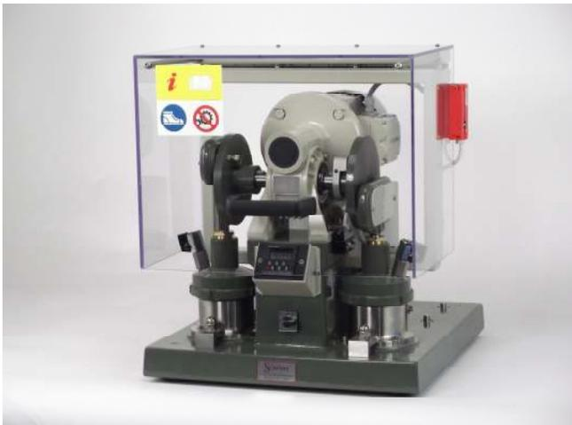
Dual-unit grease working machine
