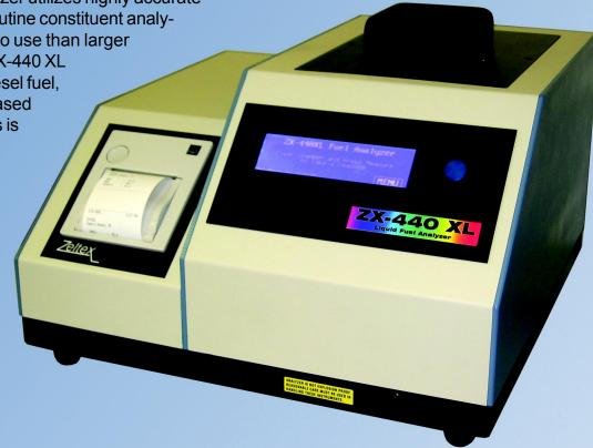
During operation, light energy that enters the liquid sample is scattered and absorbed within the sample. The ZX-440 XL analyzes the spectra exiting from the sample and directly displays the product's constituent concentrations on a large, back-lit LED display. A built-in printer provides a permanent record of test results.
