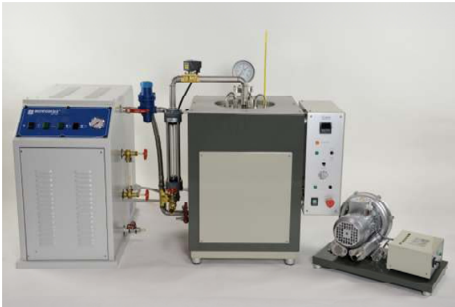
Apparatus (center) with steam generator (left) and air blower (right)
