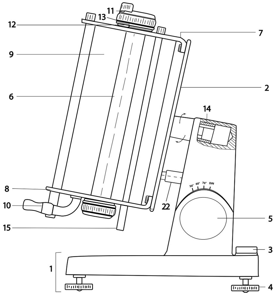
Figure 2: Falling Ball Viscometer KF10
