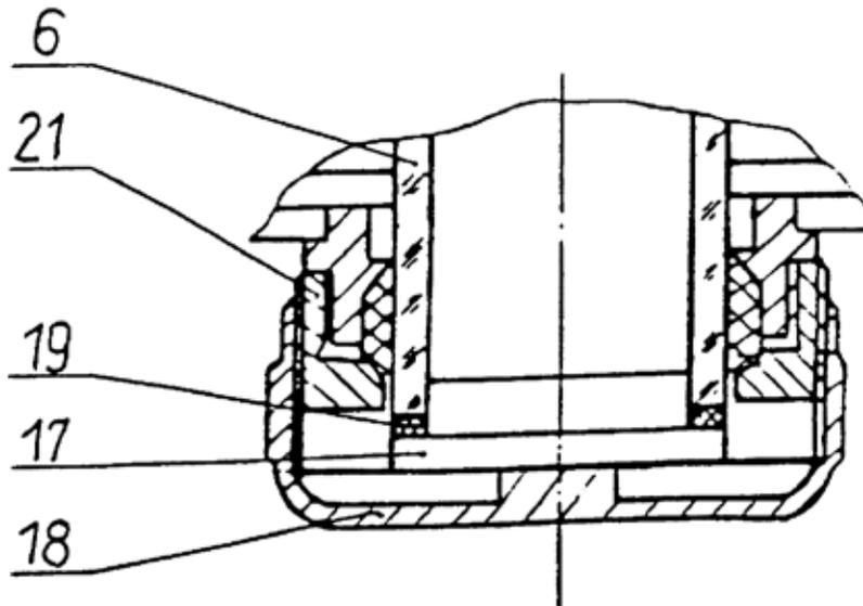
Figure 4: Sample tube screw fitting (bottom)
