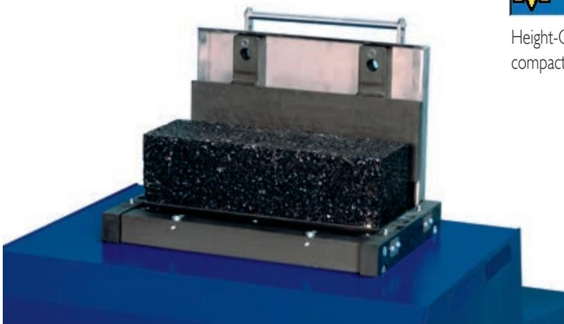
Specimen is extruded after the machine has completed the specified number of cycles, or when the required specimen height has been reached. An automatic extruder allows an easy extraction of the compacted specimen.
