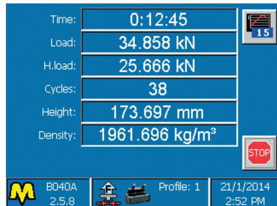
Test parameters during compaction
