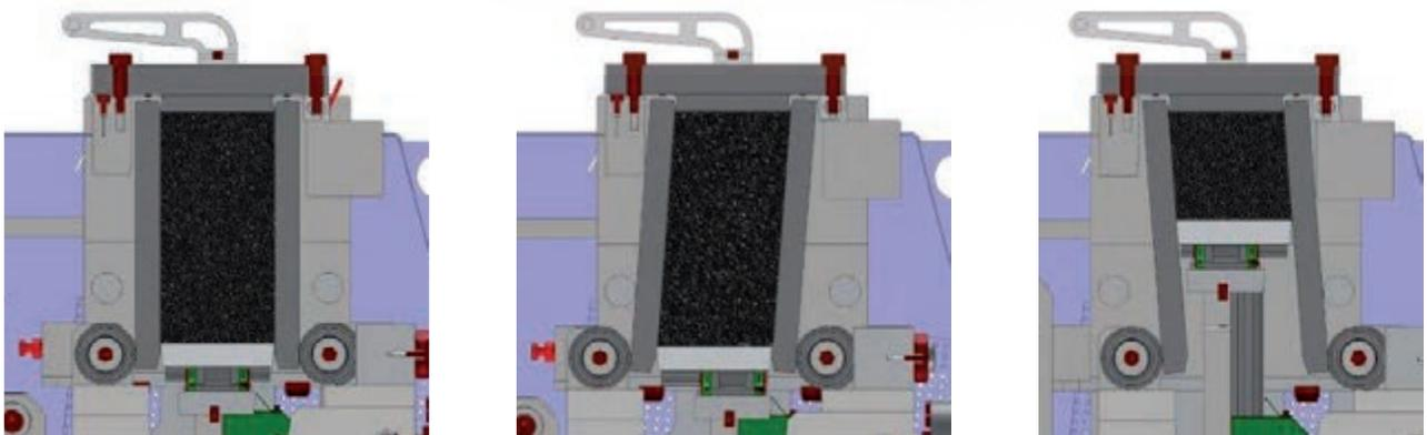
During the compaction process a lateral displacement is applied to the specimen along with a vertical load, which results in a shearing action that makes the compaction similar to the the on-field one.
