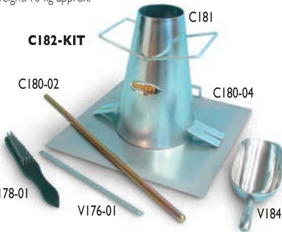
**C178-KIT** PORTABLE SLUMP CONE TEST SET, including:
