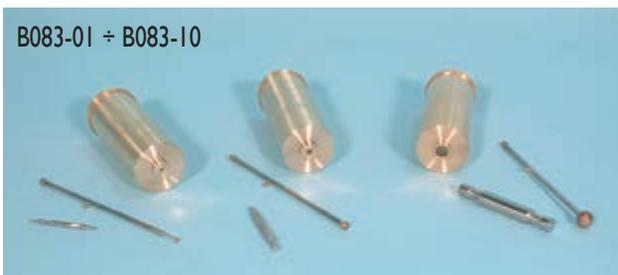
**Efflux Viscometer, "Standard TAR" (BRTA, Redwood)**
