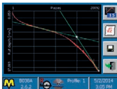
Real time results plot of the Rut Depth along with the no. of passes.
