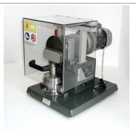
Single-unit grease working machine
