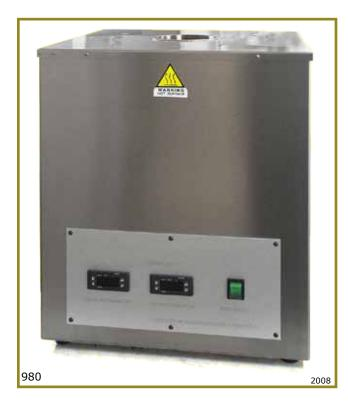
Heating block made of casting iron to 5 cells, external structure made of stainless steel, heating unit controlled by a digital thermoregulator PID with thermocouple J and overtemperature alarm., front digital thermometer with ceramic thermocouple J into a stainless steel crucible control. Cavity insulation with high efficiency.
