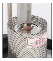
Alignment Bracket ensures concentricity of spindle and sample chamber.
