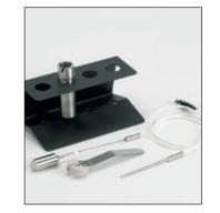
Other components supplied include sample chamber holder, RTD probe, insulating cap, coupling link, coupling nut and choice of SC4 spindle.
