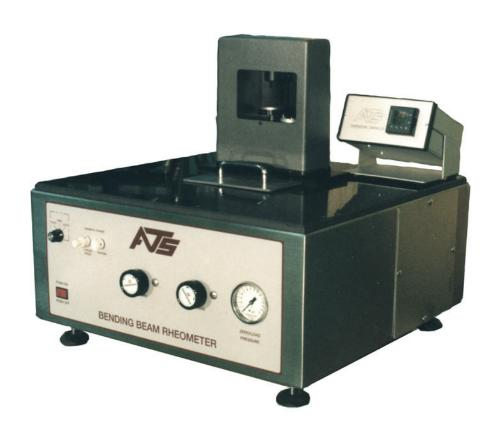
Durable, High-Quality System for Determination of Flexural Creep Stiffness of Asphalt Binder
